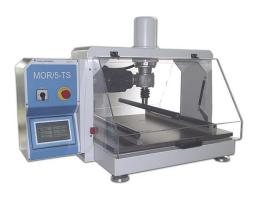
Breaking blade operated by an electro-mechanical system
