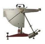
a spindle attached to a vertical pillar. At the end of the tubular arm a head of constant mass is fitted with a rubber slider. The pendulum is released from a horizontal position so that it strikes the sample surface with a constant velocity. The distance travelled by the head after striking the sample is determined by the friction of the sample surface. A reading of Skid
