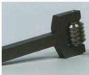
manufactured to clients' specific requirements and consists of a hardened steel barrel into which are machined a number of blades. There are two outer blades and three glaze thickness measurement blades. These are set
