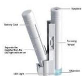
The Glaze Thickness Pocket Microscope is held against the edge of a cut piece of fired ceramics and the thickness of the glaze and also the sub surface can be easily seen under magnification.
