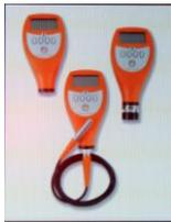
456GTM glaze thickness measuring instrument is available in any combination of Basic, Standard and Top functionality, and can be supplied with a variety of probes to suit your individual needs
