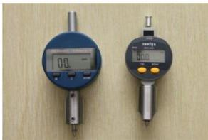
The Anderen Glaze Thickness Penetrometer has been designed to offer a simple and effective method to test the thickness of unfired glaze on ceramic surfaces.
